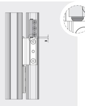
» ± 3 mm adjustement with 3 mm allen key
